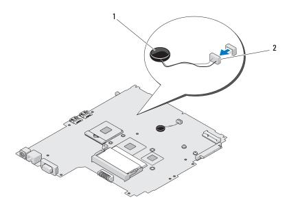
1 coin-cell battery 2 coin-cell battery cable connector
