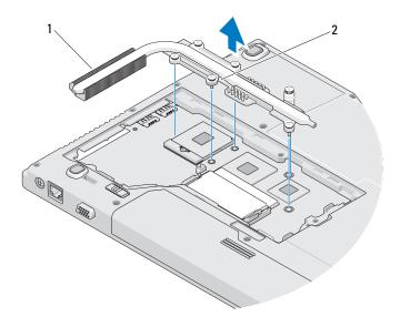
processor thermal-cooling 1 assembly
